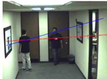
Fig. 1. Transfer of tag information via epipolar geometry
